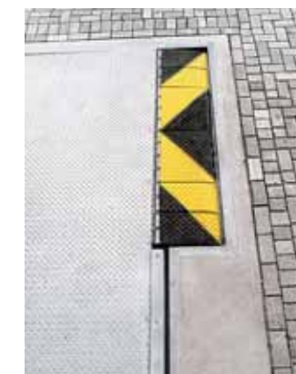
Elevating platform with a manual loading bridge that can be driven over.
