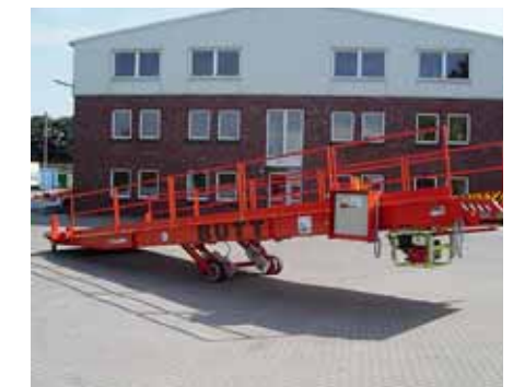
Self-propelled ramp with integrated four-stroke unit.
