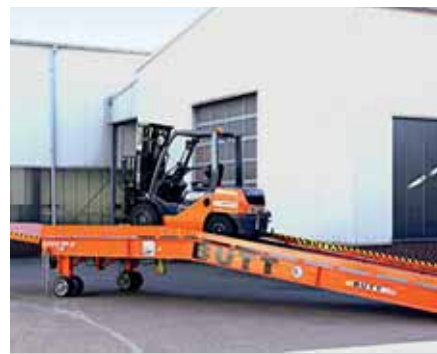
Front axle ramp with long, hydraulically operated loading bridge.
