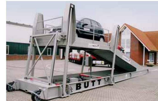
Test ramp for determining the climbing ability of hydraulic drive systems.
