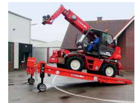
Short mobile ramp for loading construction vehicles.
