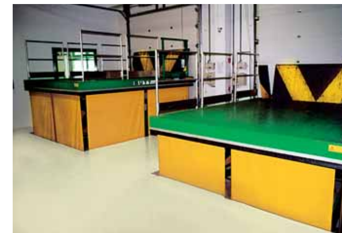
Scissor elevating platforms with various accessories. Plug railings, electrohydraulic loading bridges, underrun protective system on all sides.
