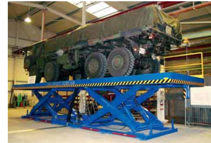
Special use for high carrying capacities for loading industrial vehicles.
