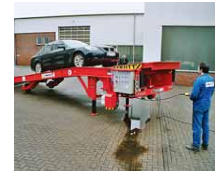
Mobile yard ramp with dock leveller and electric end carriage.
