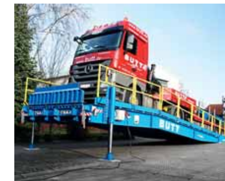
Lorry loading with electrohydraulic height adjustment.
