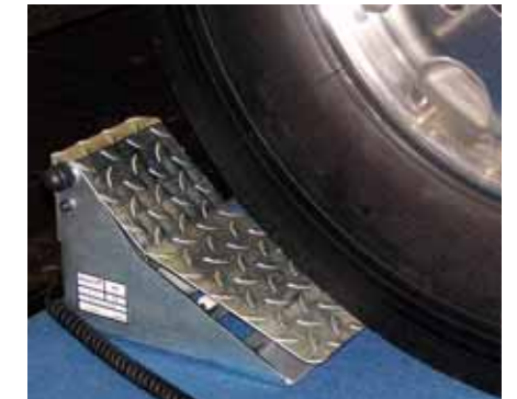
Electric BUTT safety wheel chock
