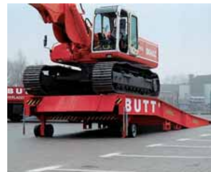
Track vehicle loading up to 42 t carrying capacity.
