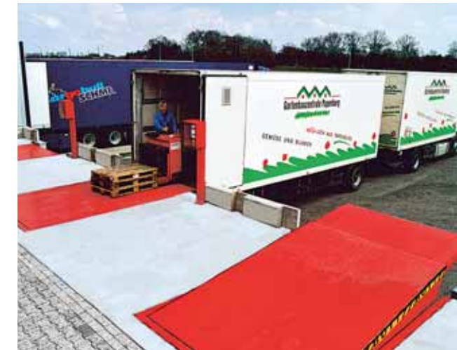
Open loading plant with weatherproof steering column and 1000 mm dock.
