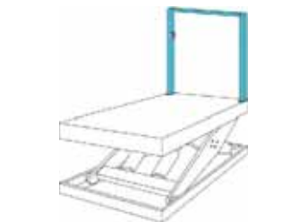
Gantry: Height depending on ramp dimensions, control device optional, steel pipe
