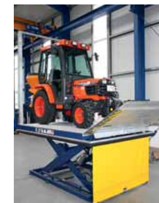
Loading table with electrohydraulic aluminium loading bridge.
